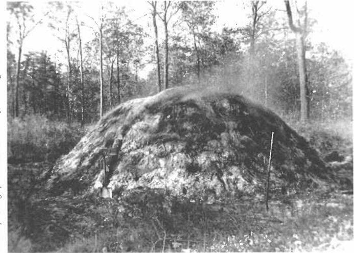
A smoldering charcoal mound. It is covered with hurdle and you can see smoke coming out of the top.
